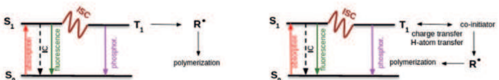
Figure 1: Polymerization mechanism for Norrish type I (left) and II (right) PIs.
