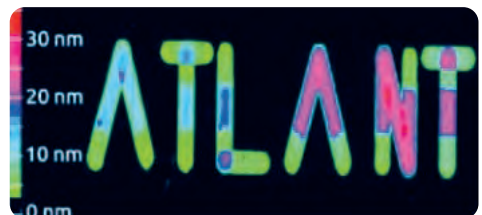
Figure: A pattern consisting of 10 to 30 nm thick platinum line segments generated by direct ALAM. Area: 12 \times 6 \text{ mm}^2 .
