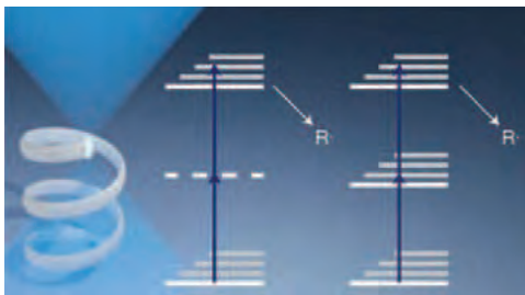
Figure 1 (taken from [1] ): Schematic illustration of the energy levels and excitation process in two-photon absorption (center) and two-step absorption (right).
