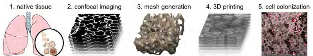
Figure 1: An excerpt of a native mouse alveoli was imaged by confocal microscopy and converted to print job instructions. These were printed using two-photon stereolithography with gelatin methacryloyl. After development, cells were seeded and cultivated on micro scaffolds in vitro . (Image adapted from [1] )
